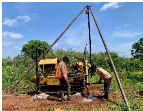
Figure 41: Core drilling machines deployed at site
