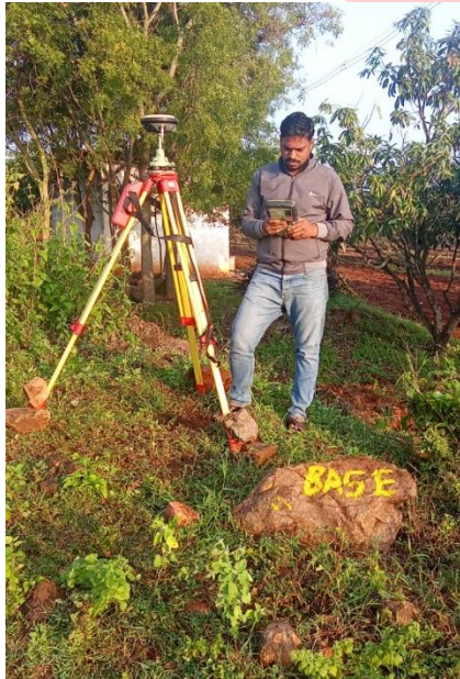
Figure 38: DGPS instrument established at Base point
