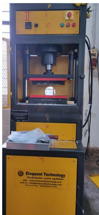
Figure 64: Hydraulic core splitting machine available at MEL, KIOCL Ltd., Mangalore.
