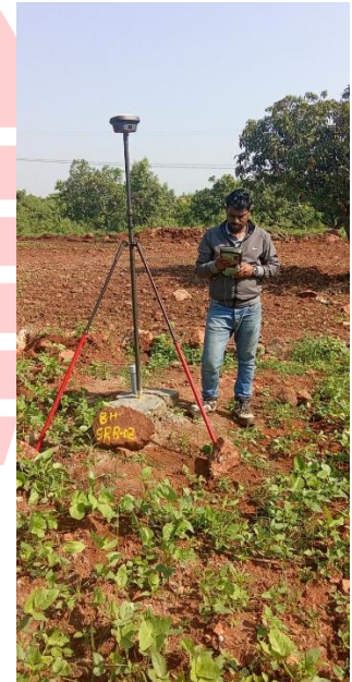
Figure 40: DGPS instrument established at Borehole 2
