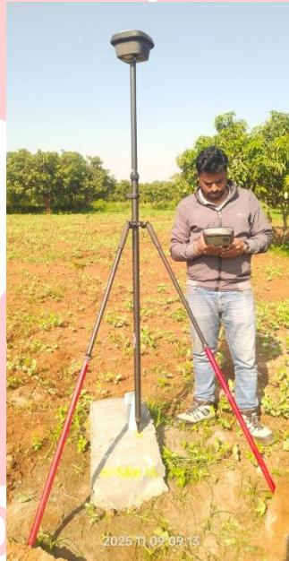
Figure 39: DGPS instrument established at Borehole 1
