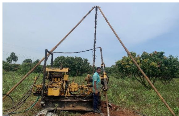
Figure 41: Core drilling machines deployed at site
